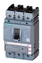
circuit breaker 3VA5 UL frame 250 breaking capacity class M 35kA @ 480 V 3-pole, line protection TM230, FTAM, In=80A overload protection Ir=80A fixed short-circuit protection li=5...10 x In cable connection on both sides
