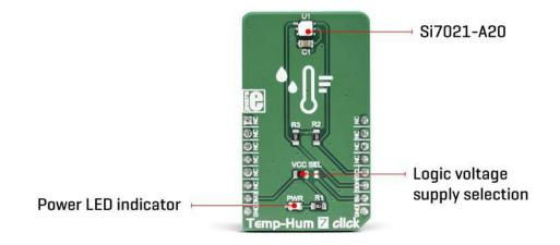
Each sensor contains the factory calibration data in the internal non-volatile memory, so there is no need for additional calibration steps. The datasheet of the Si7021-A20 offers conversion formulas, which should be used to convert the readings from the sensor to physical values, expressed in % RH and  $^{\circ}$ C.
