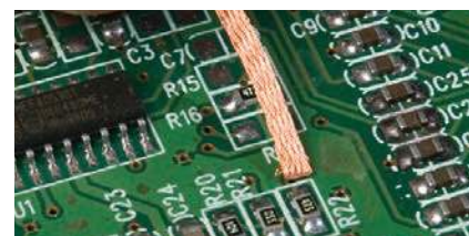
Match braid width to contact area
