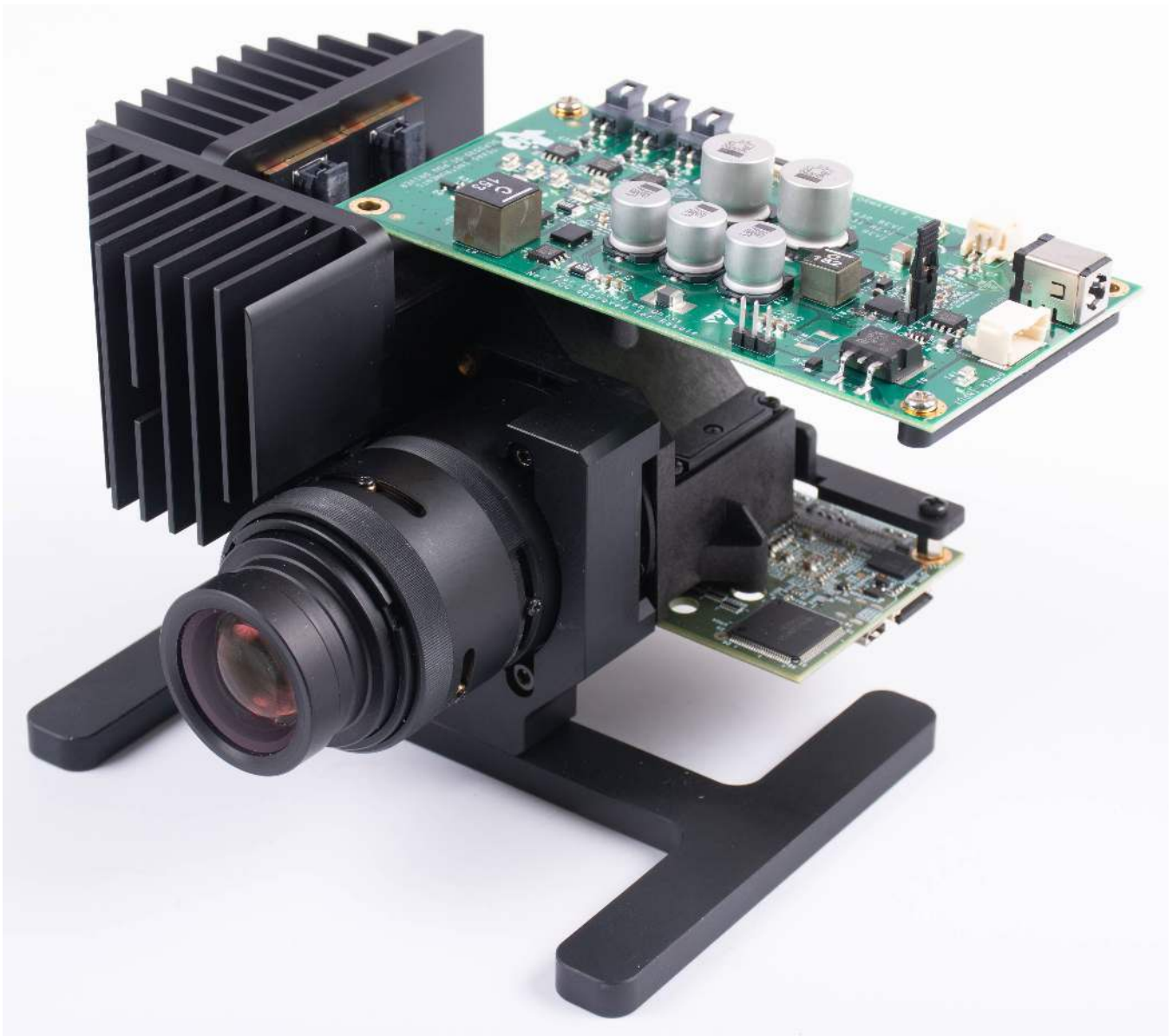
Figure 8. DLP5530PGUQ1EVM Optical Module
