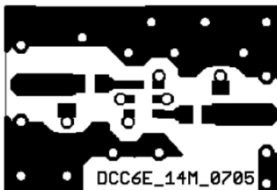
Figure 4: Optimised PCB layout for SAW filters in DCC6E package, pinning 1,4 (top side, scale 1:1).
