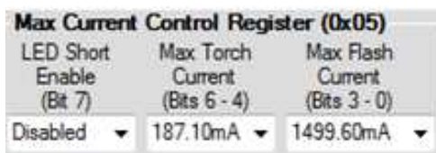
Figure 23. Max Current Control Register
