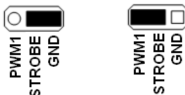
Figure 3. STROBE Jumper Settings
