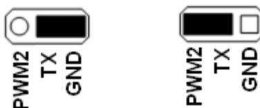
Figure 5. TX Jumper Settings
