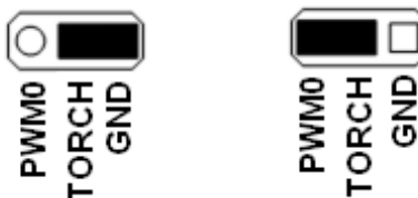
Figure 4. TORCH Jumper Settings
