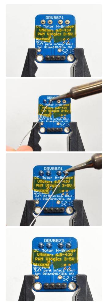
Solder in both pins of each terminal block. You can remove the tape when done.
