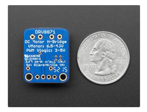
You can set the current limiting with an external resistor Rlim. We solder in a 30K resistor by default for a ~2A current limit, however you can remove this resistor and/or solder a resistor over it to change the resistance and change the limit.
