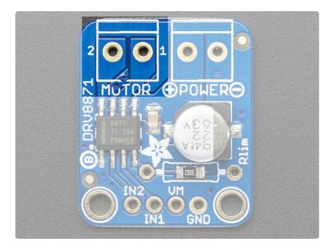
Pretty simple - this is where your motor goes! Works with any DC brushed motor. Use thick wires to avoid dropping voltage across the wire resistance
