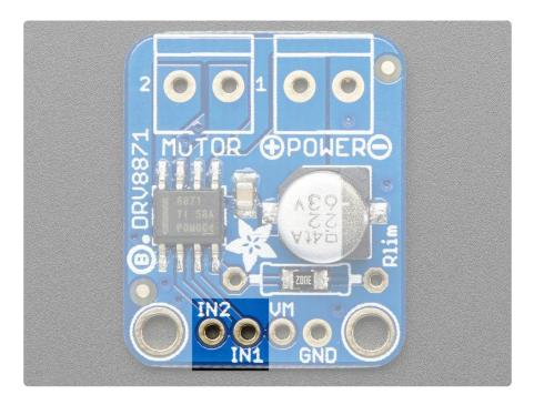
These are the inputs to the motor control. IN2 goes to OUT2, IN1 goes to OUT1. Use up to 5.5V DC logic on these pins. You can PWM the inputs up to 200KHz, but lower frequencies will be more efficient.
