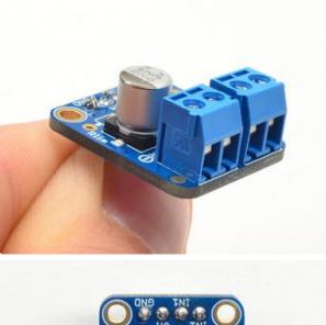
Next we will solder in the two 3.5mm terminal blocks used to connect power & the motor to the breakout board.
