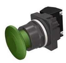
30mm BlackMax, Epoxy Coated Corrosion Resistant Complete Metal Unit Twist-to-Release Operator Non-Illuminated Mushroom Head Cap Small 1.79" (45 mm) Plastic Cap, Green 2 Position Maintained, Twist-to-Release with 1 N.O. - 1 N.C. Heavy Duty Contacts, A600/P600 UL Listed, CSA Certified NEMA 1,3,3R,4,4X,12,13 & Automotive Standards
