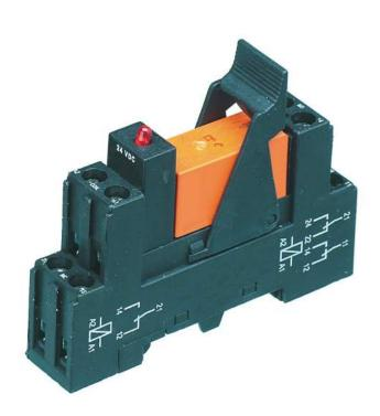
Pre-assembled relay module PRS..., Screw connection, Consisting of: relay socket base, power contact relay, pluggable display/suppression module and holding clip, 2 CO contacts, Input voltage: 60 VDC
