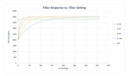
The graph above shows the effect of the filter on response times. Increasing the filter setting increases the measurement output response time.  $T_{90}$  is the time to 90% of reading. The SprintIR<sup>®</sup>-R takes 50 readings per second. The flow rate was set at 0.2l/min.
