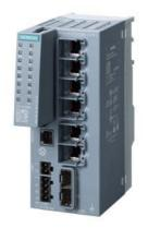
SCALANCE XC206-2SFP G (E/IP) manageable Layer 2 IE switch; IEC 62443-4-2 certified; 6x 10/100/1000 Mbit/s RJ45 ports; 2x 1000 Mbit/s SFP; 1x console port; diagnostics LED; redundant power supply; temperature range -40 °C to +70 °C; assembly: DIN rail/S7 mounting rail/wall; redundancy functions; office features (RSTP, VLAN,...); PROFINET IO device; Ethernet/IP-compliant; C-PLUG slot; default EtherNet/IP.
