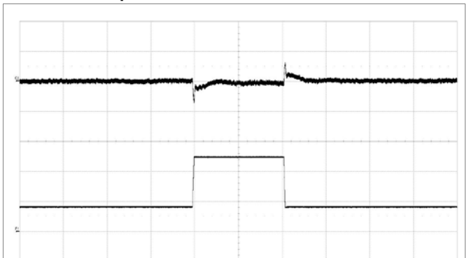
Output voltage response to load current step change (25%–75%–25%) at V_I = 12\text{ V} , C_{OUT} = 8 \times 330\text{ }\mu\text{F}/10\text{ m}\Omega + 20 \times 100\text{ }\mu\text{F} , di/dt = 2\text{ A}/\mu\text{s} , ACSR\text{ Gain}=219 and ASCR\text{ Residual}=82 . Scale from top: 50 mV/div, 20 A/div, 500 \mu\text{s} /div. Note: Sense pins are connected to load.
