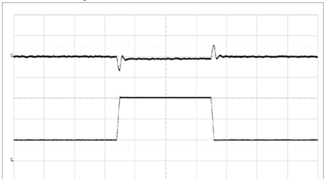
Output voltage response to load current step change (25%–75%–25%) at V_I = 12\text{ V} , C_{OUT} = 8 \times 330\text{ }\mu\text{F}/10\text{ m}\Omega + 20 \times 100\text{ }\mu\text{F} , di/dt = 2\text{ A}/\mu\text{s} , ACSR Gian=219 and ASCR Residual=82. Scale from top: 50 mV/div, 20 A/div, 200 \mu\text{s}/\text{div} . Note: Sense pins are connected to load.
