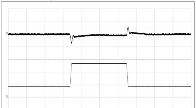
Output voltage response to load current step change (25%–75%–25%) at V_I = 12\text{ V} , C_{OUT} = 8 \times 330\text{ }\mu\text{F}/10\text{ m}\Omega + 20 \times 100\text{ }\mu\text{F} , di/dt = 2\text{ A}/\mu\text{s} , ACSR\text{ Gian}=219 and ASCR\text{ Residual}=82 . Scale from top: 50 mV/div, 20 A/div, 200 \mu\text{s} /div. Note: Sense pins are connected to load.
