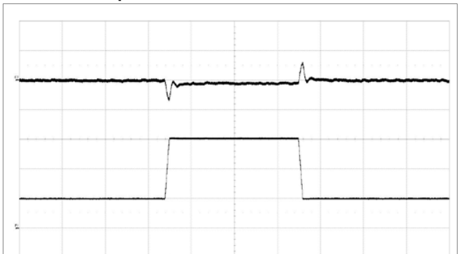
Output voltage response to load current step change (25%–75%–25%) at V_I = 12\text{ V} , C_{OUT} = 8 \times 330\text{ }\mu\text{F}/10\text{ m}\Omega + 20 \times 100\text{ }\mu\text{F} , di/dt = 2\text{ A}/\mu\text{s} , ACSR Gian=219 and ASCR Residual=82. Scale from top: 50 mV/div, 20 A/div, 200 \mu\text{s} /div. Note: Sense pins are connected to load.
