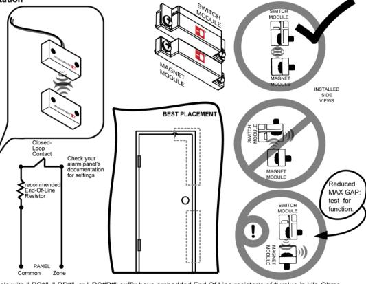
Models with "-RS#", "-RP#", or "-RS#P#" suffix have embedded End Of Line resistor/s of # value in kilo-Ohms.
