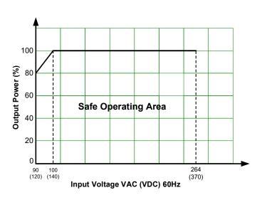
Note: With an AC input voltage between 90-100VAC and a DC input between 120-140VDC the output power must be derated as per the temperature derating curves.
