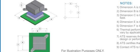
1) Dimension A is the length of the heat sink in the direction of the flow. 2) Dimension B is the width of the heat sink perpendicular to the flow direction.
