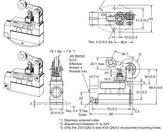
Note: Unless otherwise specified, a tolerance of  $\pm 0.4$  mm applies to all dimensions.
