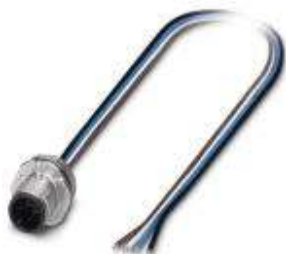
Sensor/actuator sealed flush-type connector, 4-pos., M12 SPEEDCON, A-encoded, front/screw mounting with M16 thread, with 0.5 m TPE litz wire, 4 x 0.34 mm 2
