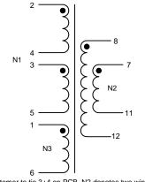
Customer to tie 3+4 on PCB. N2 denotes two windings connected in parallel. Terminals 7+8, 11+12 must be tied as solder bridging is allowed.
