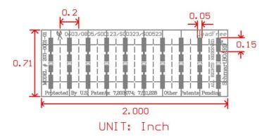
203-0001-01 4 Pack of SchmartPatch for 0603, 0805, SOD123, SOD323 and SOD523
