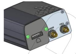
Use the two Pan-Head screws supplied with the IoT card to screw the end-plate into place.
