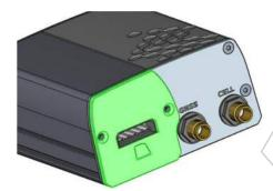
Place the replacement end-plate (supplied with the IoT card) over the end of the connector on the IoT card and line up the two screw holes.
