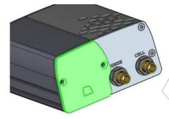
Once both screws have been removed, take the original end-plate off the FX30 and set it aside.
