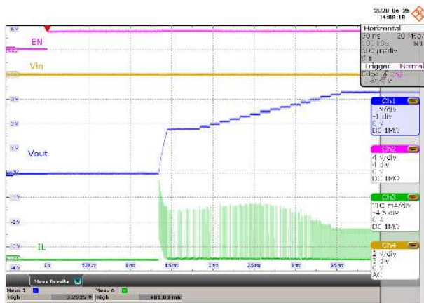
Figure 8-26. Load Transient, 300 mA Step
