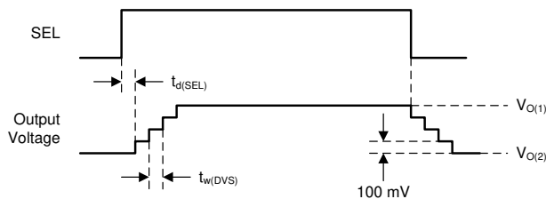
Figure 7-10. Dynamic Voltage Scaling with High Load
