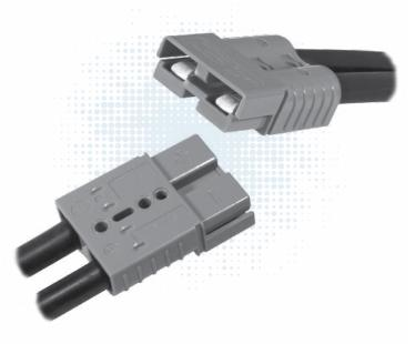
Like the other Multipole connectors, the SB<sup>®</sup>120 offers color-coded mechanically keyed housings. Keys can be used to identify and separate different circuits, or prevent users from accidentally cross mating different voltages. Wires sizes from #10 ( $5.3 \text{ mm}^2$ ) to #1 ( $42.4 \text{ mm}^2$ ) are held in the second smallest SB<sup>®</sup> housing.
