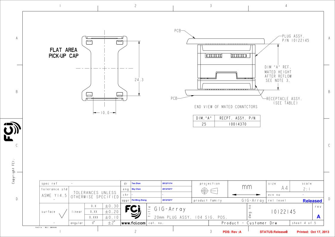
HOUSING: LCP UL RATING: 94 V-O CONTACT: COPPER ALLOY PLATING (CONTACT): Au OVER Ni. SOLDER BALL: (SEE TABLE) EUTECTIC SnPb OR LEADFREE 95.5 Sn/4Aq/0.5Cu
