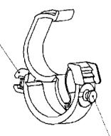
Ø5mm "T" stud Interconnecting mâle device /
