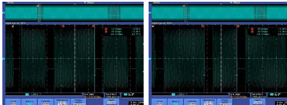
Figure 6-31. Receive Data Bits and Framing Level
