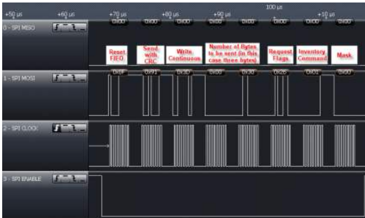
Figure 6-22. Inventory Command Sent From MCU to TRF7964A
