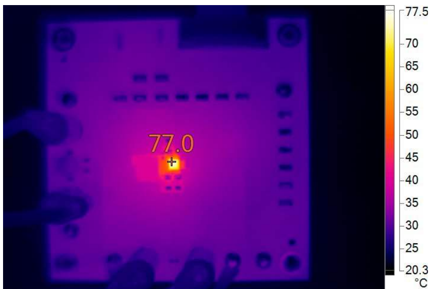
Figure 7. Thermal Image of DC3145A
