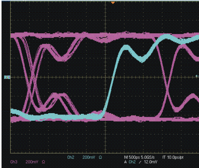
Figure 104. LVDS Eye Diagram - No Internal Termination 5-pF Load Capacitance Blue Trace - Output Clock (CLKOUT) Pink Trace - Output Data
