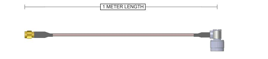
Connector A 132195 SMA Plug Straight Brass Gold + Heatshrink 50 Ohm RG-142 Continuity/Hi-Pot
