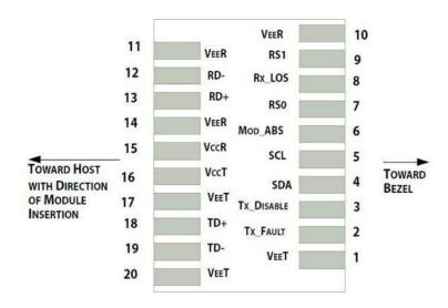
Pin-out of connector Block on Host board
