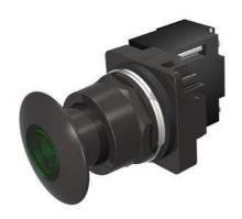
30mm BlackMax, Epoxy Coated Corrosion Resistant Complete Metal Unit Illuminated Push-Pull Operator Full Voltage, 6V AC LED Lamp Mushroom Head Cap Small 1 3/4" (44.5 mm) Metal, Black with Green Lens 3 Position Pull-Momentary/Push-Maintained UL Listed, CSA Certified NEMA 1,3,3R,4,4X,12,13 & Automotive Standards
