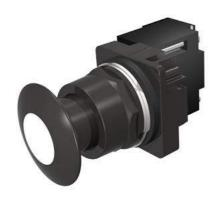
30mm BlackMax, Epoxy Coated Corrosion Resistant Complete Metal Unit Illuminated Push-Pull Operator Transformer type, 120V AC Incandescent Lamp Mushroom Head Cap Small 1 3/4" (44.5 mm) Metal, Black with White Lens 3 Position Momentary UL Listed, CSA Certified NEMA 1,3,3R,4,4X,12,13 & Automotive Standards
