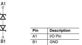
Due to the symmetrical configuration no marking information is needed.
