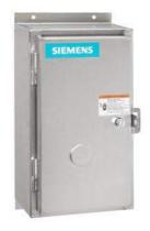
Non-reversing NEMA contactor, Size 2, Three phase full voltage, Contactor amp rating 45A, 3 wire (NO aux included), 220-240/440-480VAC 60Hz coil, Non-combination type, Encl NEMA type 4X 304 S-Steel, Water/dust tight noncorrosive, Standard width enclosure
