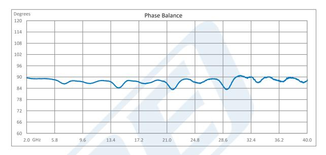
90 Degree 2.92mm Hybrid Coupler from 2 GHz to 40 GHz Rated to 20 Watts from Pasternack Enterprises has same day shipment for domestic and International orders. Our RF, microwave and millimeter wave products maintain a 99.4% availability and are part of the broadest selection in the industry.
