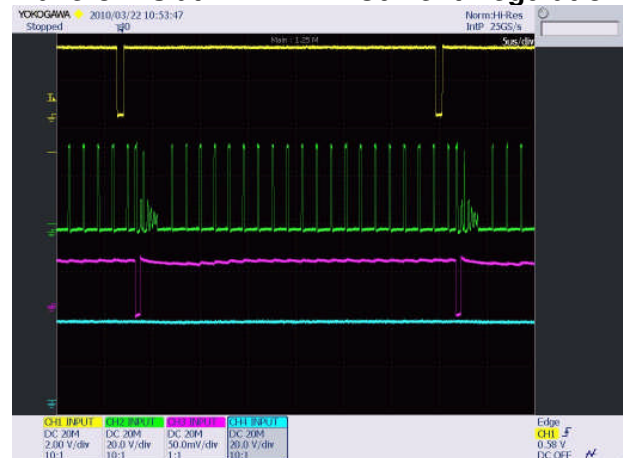
Ch 1 (yellow) – PWM signal at 30 kHz 98% duty cycle Ch 2 (green) – SW node voltage, Ch 3 (red) – LED Current. Ch 4 (blue) - V_{OUT}
