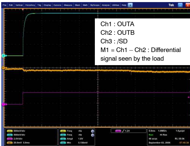
Figure 25. Zero pop noise turn on sequence with single-ended input to ground ( C_i = 100 \text{ nF} , R_i = 24 \text{ k}\Omega , R_f = 24 \text{ k}\Omega , C_{byp} = 1 \text{ }\mu\text{F} , R_l = 8 \text{ }\Omega , T_{on} = \text{GND} )
