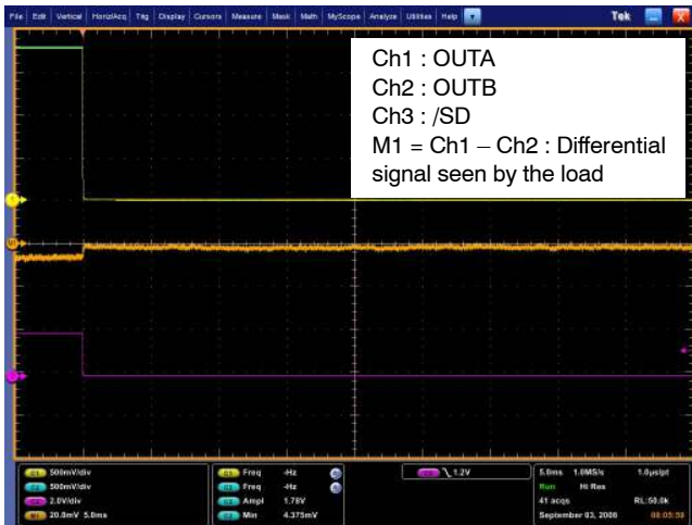
Figure 39. Zero pop noise turn off sequence with differential input to ground ( C_i = 47 \text{ nF} , R_i = 24 \text{ k}\Omega , R_f = 24 \text{ k}\Omega , C_{\text{byp}} = 1 \text{ }\mu\text{F} , R_l = 8 \text{ }\Omega , T_{\text{on}} = V_p )
