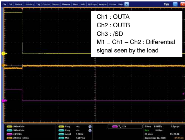
Figure 27. Zero pop noise turn off sequence with single-ended input to ground ( C_i = 100 \text{ nF} , R_i = 24 \text{ k}\Omega , R_f = 24 \text{ k}\Omega , C_{byp} = 1 \text{ }\mu\text{F} , R_l = 8 \text{ }\Omega , T_{on} = \text{GND} )
