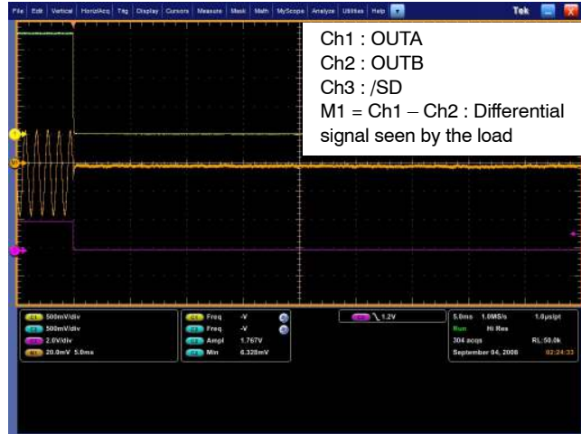
Figure 36. Zero pop noise turn off sequence with single-ended input audio source ( C_i = 47 \text{ nF} , R_i = 24 \text{ k}\Omega , R_f = 24 \text{ k}\Omega , C_{\text{byp}} = 1 \text{ }\mu\text{F} , R_l = 8 \text{ }\Omega , T_{\text{on}} = V_p )
