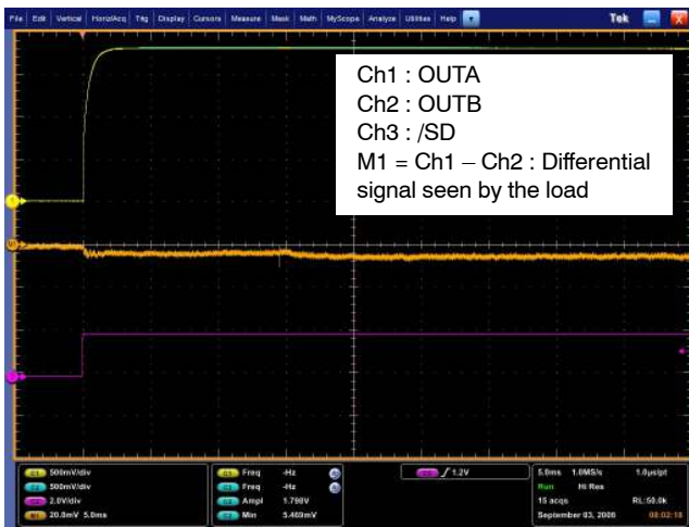
Figure 33. Zero pop noise turn on sequence with single-ended input to ground ( C_i = 47 \text{ nF} , R_i = 24 \text{ k}\Omega , R_f = 24 \text{ k}\Omega , C_{\text{byp}} = 1 \text{ }\mu\text{F} , R_l = 8 \text{ }\Omega , T_{\text{on}} = V_p )
