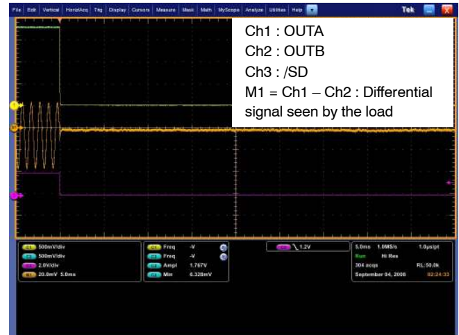
Figure 28. Zero pop noise turn off sequence with single-ended input audio source ( C_i = 100 \text{ nF} , R_i = 24 \text{ k}\Omega , R_f = 24 \text{ k}\Omega , C_{byp} = 1 \text{ }\mu\text{F} , R_l = 8 \text{ }\Omega , T_{on} = \text{GND} )
