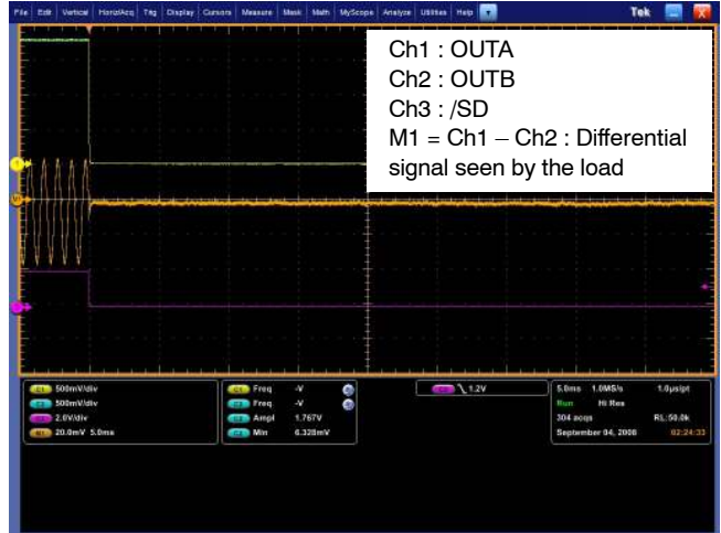
Figure 32. Zero pop noise turn off sequence with differential input audio source ( C_i = 100 \text{ nF} , R_i = 24 \text{ k}\Omega , R_f = 24 \text{ k}\Omega , C_{\text{byp}} = 1 \text{ }\mu\text{F} , R_l = 8 \text{ }\Omega , T_{\text{on}} = \text{GND} )
