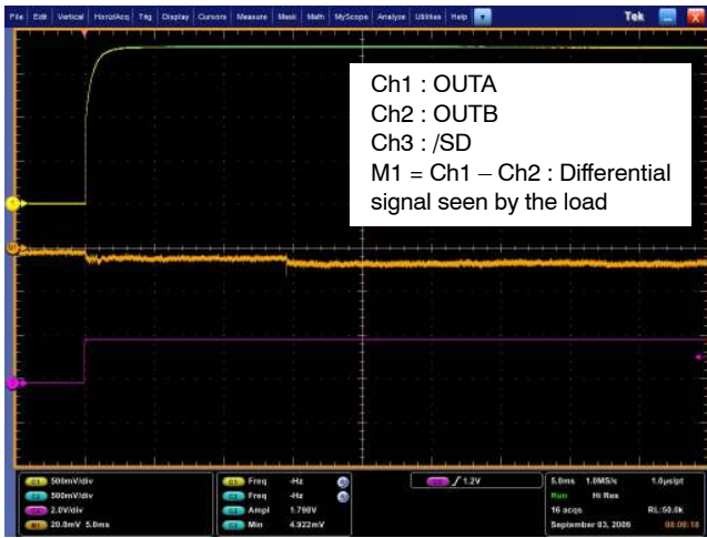
Figure 37. Zero pop noise turn on sequence with differential input to ground ( C_i = 47 \text{ nF} , R_i = 24 \text{ k}\Omega , R_f = 24 \text{ k}\Omega , C_{\text{byp}} = 1 \text{ }\mu\text{F} , R_l = 8 \text{ }\Omega , T_{\text{on}} = V_p )
