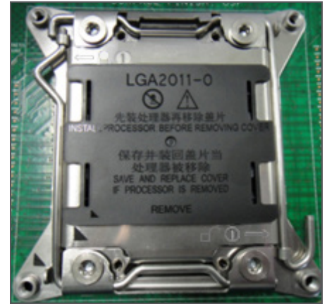
LGA 2011-0 CPU Socket with Standard Independent Loading Mechanism (ILM) and (optional) ILM cover
