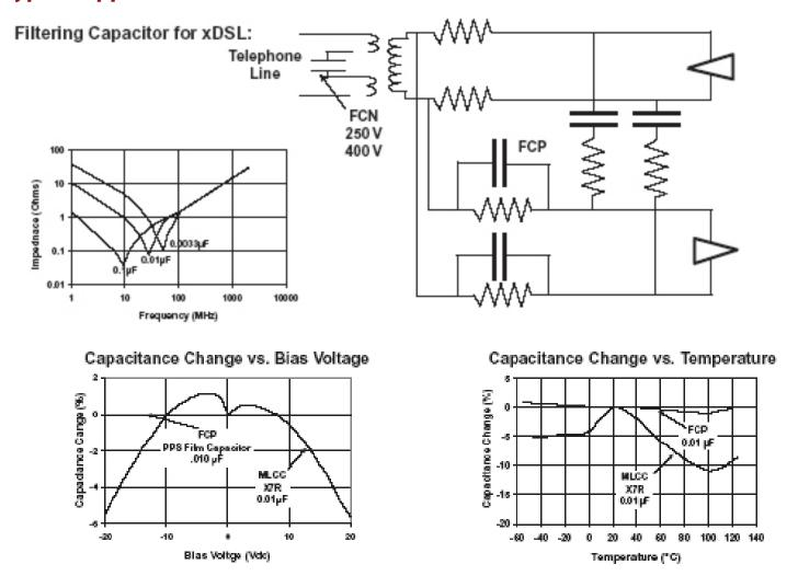
The capacitance of SMT film chips is much more stable with applied voltage and with changes in temperature than multilayer ceramic capacitors. Add in the low ESR characteristics of film chips and the final result is improved performance in filter circuit applications.
