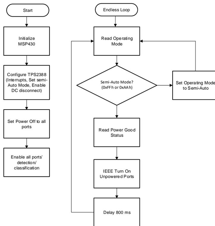
Figure 12. Virtual Auto Mode Reference Code Structure
