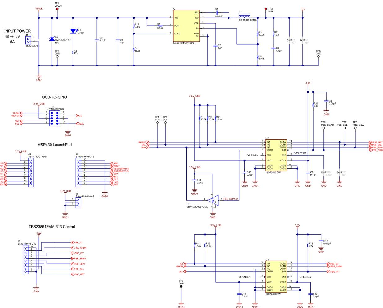
Figure 15. TPS2388EVM-612 (Motherboard) Schematic: Control
