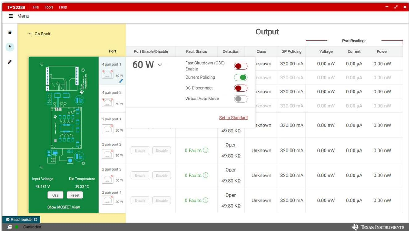
Figure 6. Device Configuration and Telemetry Page With Edit
