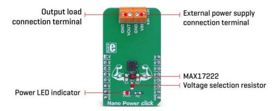
Operation of the MAX17222 changes with the connected load, as mentioned above. When the load is very light, the device operates in the Ultra Low Power Mode (ULPM) and the switching is performed in discontinuous mode (DCM). The ULPM is typically used when the device connected at the output is in standby or power down mode, draining a very low amount of current. As the current requirement increases, the MAX17222 device switches to the Low Power mode and further to the High Power
