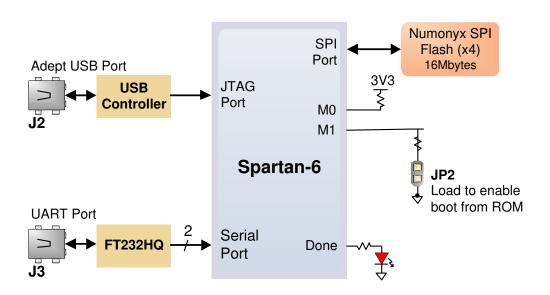
An on-board mode jumper (JP2) selects between JTAG/USB and ROM programming modes. If JP2 is loaded, the FPGA will automatically configure itself from the ROM. If JP2 is not loaded, the FPGA will remain idle after power-on until configured from the JTAG port.
