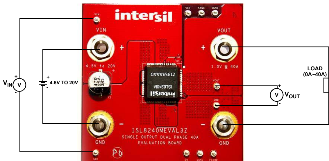
FIGURE 1. ISL8240MEVAL3Z BOARD IMAGE
