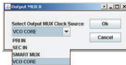
Figure 8. Output MUX (each output channel)
