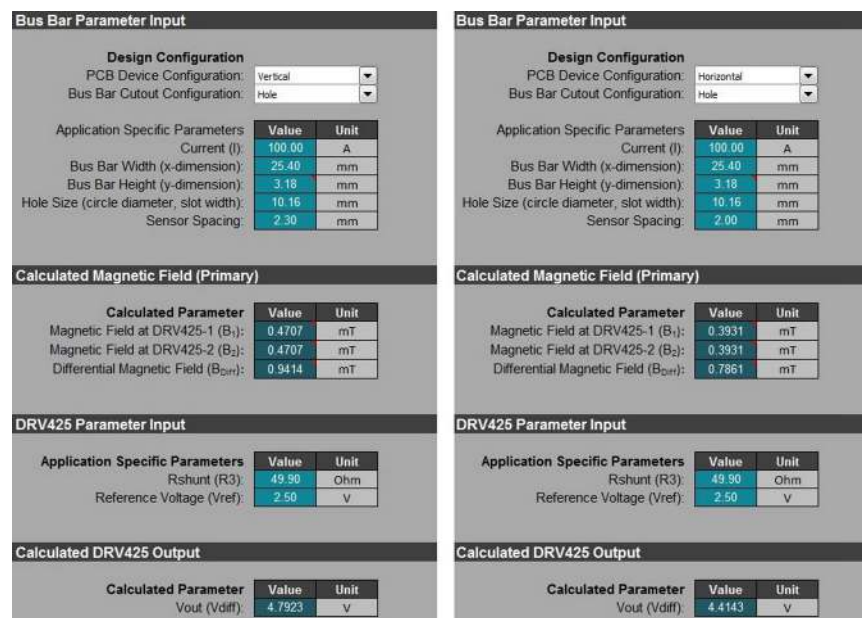
Figure 2. DRV425 Busbar Application Magnetic Field Calculator for Vertical and Horizontal Design
