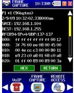
Capture up to 10,000 packets for analysis including packet size, source and destination IP address, time detected and packet type. User defined filters capture specific data needed to identify problems and monitor performance.
