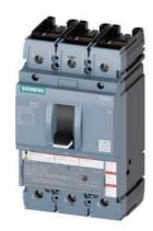
circuit breaker 3VA5 UL frame 250 breaking capacity class C 100kA @ 480 V 3-pole, line protection TM210, FTFM, In=200A overload protection Ir=200 A fixed short-circuit protection Ii=10 x In UL489 SB (naval), 50 deg. cel. cable connection on both sides
