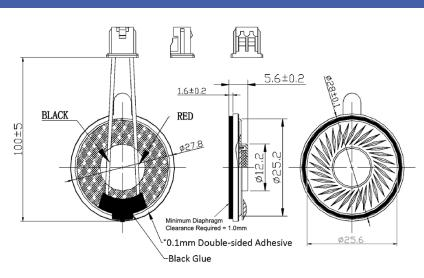
General tolerance =  $\pm 0.5$  mm and all measurements in mm unless otherwise noted.
