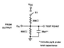
This is the A.C. Test Load which Harris Semiconductor uses in its automatic test equipment, and it is recommended that users of Harris bipolar devices use the same or an equivalent load in performing A.C. testing.
