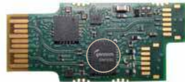
Rx CDR+ Tx Burst Mode DML driver GN7355 - Symmetric PON GN7354 - Asymmetric PON
