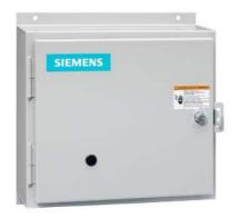
Non-reversing NEMA contactor, Size 1, 4 power poles, Contactor amp rating 27A, 3 wire (NO aux included), 110V 50Hz / 120V 60Hz coil, Non-combination type, Enclosure NEMA type 12, Dust/drip proof for indoors, Standard width enclosure
